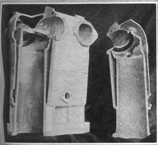
Sawn-up section of large aluminum motor for aeroplane work. The dark rings are the cast iron valve seats which were given a thin coat of copper before making the casting so that the aluminum and iron have become almost welded together
